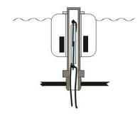
Upside Down Mounting: When the fluid switch is mounted upside down, Normally Open becomes Normally Closed and vice versa
