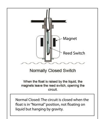
A glass reed switch is hermeticaly sealed inside the stem from the liquid environment.
